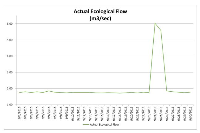
The graph above shows the actual ecological flow data the amount of water left to the Paravani River from Paravani HEPP between for September 2015. The minimum permitted ecological flow of Paravani HEPP is 1,75 m3/sec.
