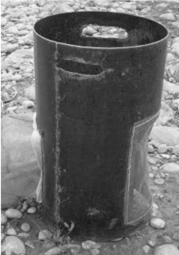
Cylindrical Bathometer of Sadovksy Height – 0.5 m Diameter – 0.3 m
