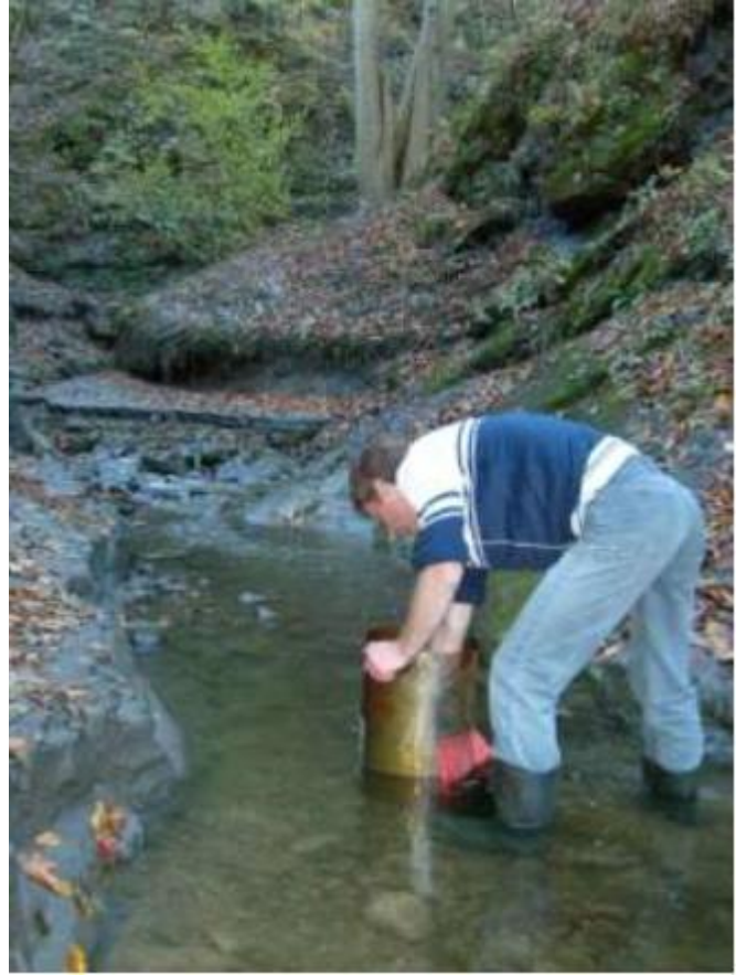
The principle of working with bathometer in the field.
